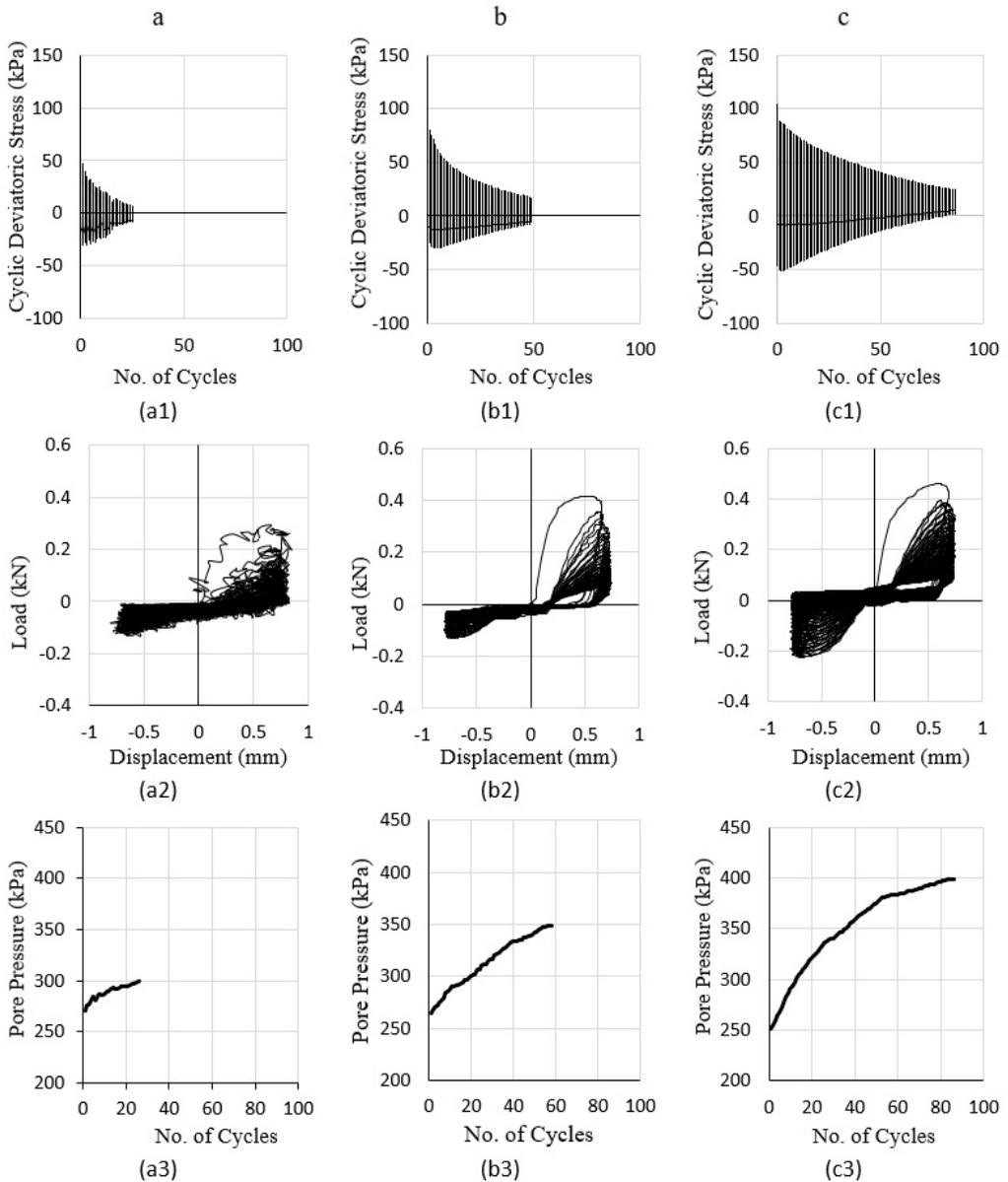
of cycles at failure also increases to initiate the liquefaction. It clearly signifies that possibility of liquefaction gets reduced with the increase in relative density of soil.
